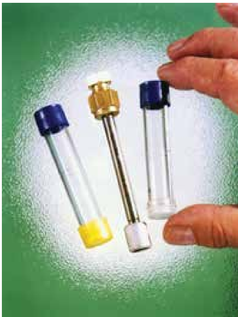
Figure 1: Diffusion Tubes for Various Pollutants from left to right: SO 2 tube ( not used in this study ), BTEX tube (centre), and NO 2 tube.
